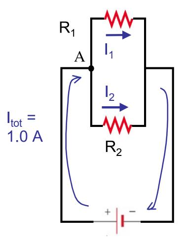
Confirm that the amount of the voltage drop across each resistor is 2V:
