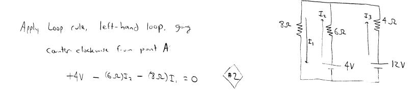
Alternate loop rule: Right-hand loop, going Counter-clockwise
