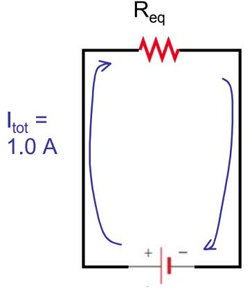
Now, calculate  $\varepsilon$  of the battery.  $1/R_{eq} = 1/(3\Omega) + 1/(6\Omega) = 1/(2\Omega)$   $R_{eq} = 2\Omega$ Loop rule for simplified circuit:  $\varepsilon = I_{tot} R_{eq} = 1.0 \text{ A } 2\Omega = 2.0 \text{ V}$
