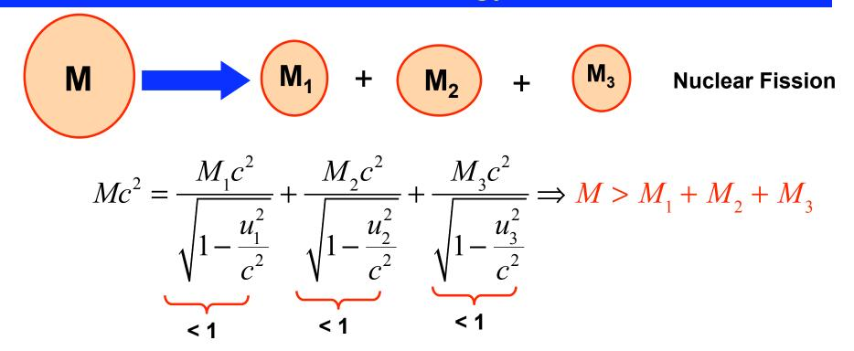
Loss of mass shows up as kinetic energy of final state particles Disintegration energy per fission  $Q=(M - (M_1+M_2+M_3))c^2 = \Delta Mc^2$
