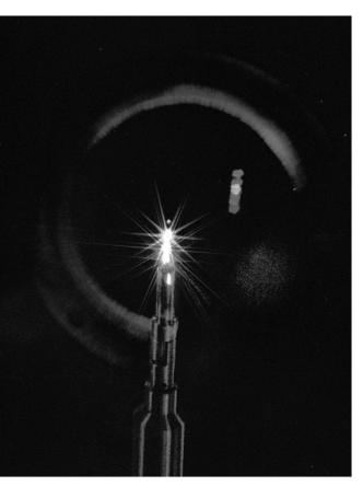
10 laser beams converge onto H pellet (0.5mm diam)
