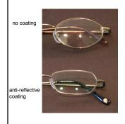
Anti-reflective coatings are used to reduce reflections at the air-glass interface
