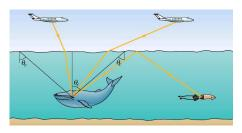
At angles greater than the critical angle the whale sees only reflected light This illustrates the point that the path of light rays is the same in the forward and reverse directions.
