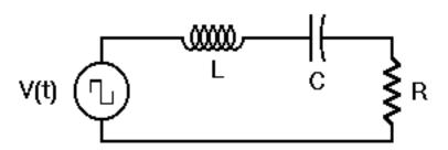
Figure 1 LRC circuit for this experiment
