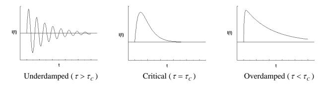
**Figure 3** *Three régimes for damping behavior.*
