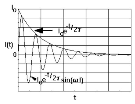
**Figure 4** Exponentially underdamped current I(t) with envelope defined by time constant  $\tau = \frac{L}{R}$ .
