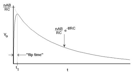
the output voltage for a flip coil moved rapidly out of a magnetic field region and integrated by an RC circuit followed by discharge of the capacitor
