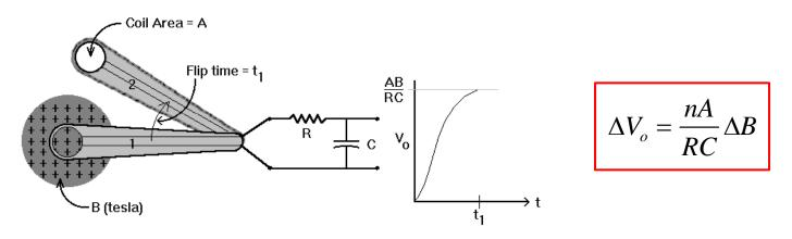
after the "flip" has occurred and the integrator output voltage has jumped to  $\Delta V_o$
