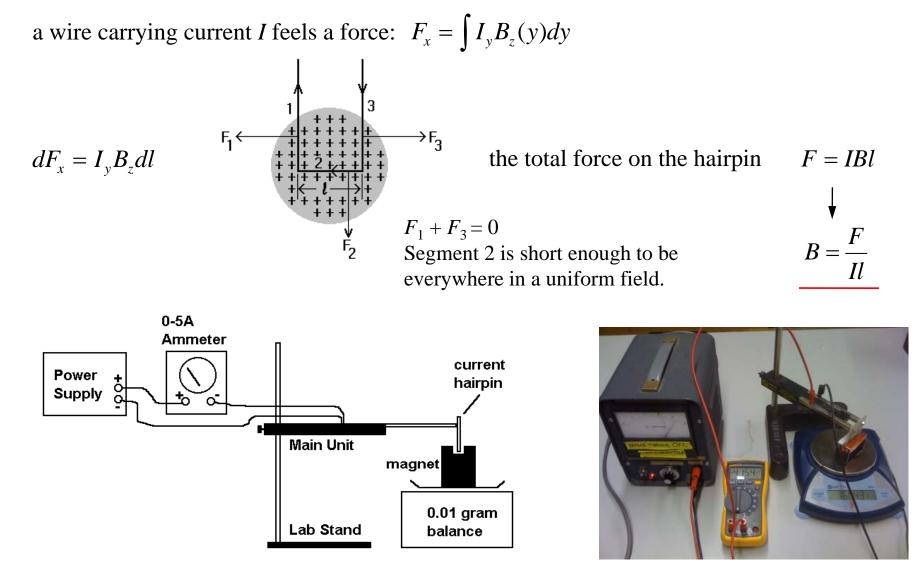
Determine the magnetic field of the magnet by measuring the force on a current in the field. Choose several hairpins of different lengths. For each hairpin choose several different currents. Measure the mass difference from the scale and calculate the Lorentz force.
