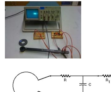
actual decay time constant is  $R_2C$ , where  $R_2 = \frac{R_1R}{R_1 + R}$ keep the flip time  $t_1$  small ( $t_1 << R_2C$ )
