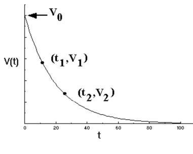
$$V_{1} = V_{0}e^{-t_{1}/\tau} \text{ and } V_{2} = V_{0}e^{-t_{2}/\tau}$$
