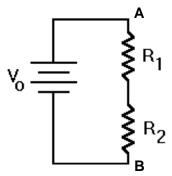
resistors  $R_1$  and  $R_2$  in series
