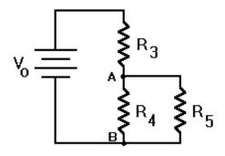
resistors R<sub>4</sub> and R<sub>5</sub> in parallel
