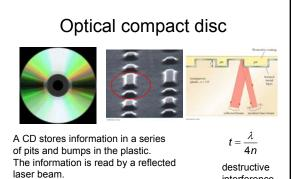
The intensity of the beam is changed by destructive interference of the reflected light interference
