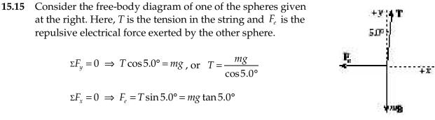
At equilibrium, the distance separating the two spheres is  $r = 2L \sin 5.0^\circ$ .
