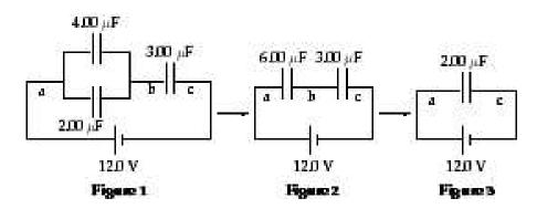
(b) From Figure 3:  $Q_{ac} = C_{ac} (\Delta V)_{ac} = (2.00 \ \mu \text{F}) (12.0 \text{ V}) = 24.0 \ \mu \text{C}$
