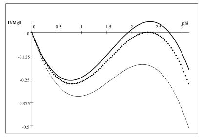
If the system is released from  $\phi = 0$  for the case m/M = .7, the wheel passes through equilibrium and comes to rest at  $\phi \approx 1.9 rad$  and returns to  $\phi = 0$ . For a heavier m, m/M = .8, the wheel passes through equilibrium and passes over the top,  $\phi = \pi$ , and continues on.
