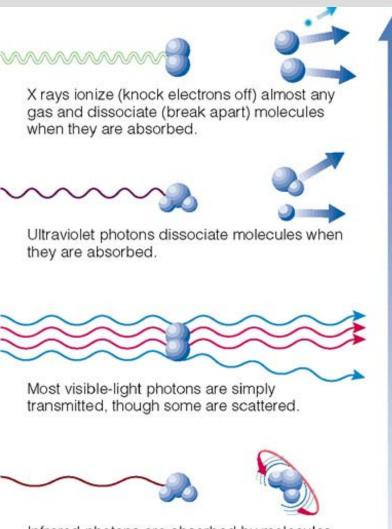
Infrared photons are absorbed by molecules, causing them to vibrate and rotate.
