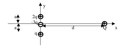
In the figure, charge 2q is at y=a, charge q is at y=-a and charge -3q is at y=0. All are at x=0. Charge Q is at y=0, x=d. The distance d>>a.
