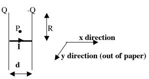
A capacitor with circular plates of radius R and distance between the plates d is discharged by connecting the centers of the plates with a straight conducting wire as shown in the figure. The point P is at distance R/10 from the axis in the center of the gap between the capacitor plates. Q>0. I>0 denotes the <u>magnitude</u> of the current. (a) Give an expression for the electric field at point P in terms of the charge on the capacitor plates Q, R, and d.
