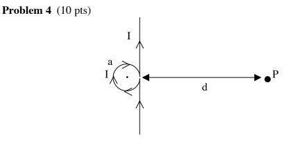
A long wire carrying current I is bent into the shape shown. The loop has radius a. (a) Find the magnitude and direction of the magnetic field at the center of the loop. (b) Find the magnitude and direction of the magnetic field at point P at distance d from the wire (P is on a line perpendicular to the wire that goes through the center of the loop). Assume d>>a, but don't ignore the contribution from the loop.
