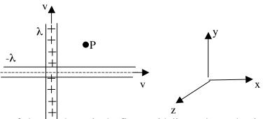
Consider the perpendicular lines of charges shown in the figure with linear charge density  $\lambda$  and  $-\lambda$ , with  $\lambda$ =12esu/cm. The lines cross at the origin of the x,y,z coordinate system and the point P is at (x,y,z)=(4cm,4cm,0).
