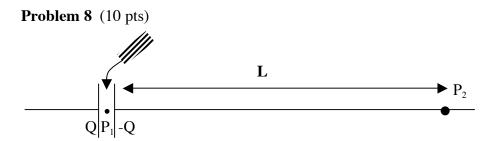
The parallel plate capacitor shown in the figure has square plates of side length a and distance between plates d, with a>>d. It has charge Q and -Q on the left and right plate respectively and is not connected to any voltage source. The point P is at distance L from the capacitor as shown in the figure, with L>>a (and L>>d).
