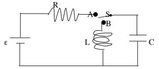
In the circuit in the figure,  $\varepsilon = 5V$ , R=2 $\Omega$ , C=3 $\mu$ F, L=4mH. Initially the capacitor C is uncharged and the circuits are open. At time t=0, the switch S is connected to point A. (a) Find the current through the resistor  $I_R(t)$  as function of time and plot it.
