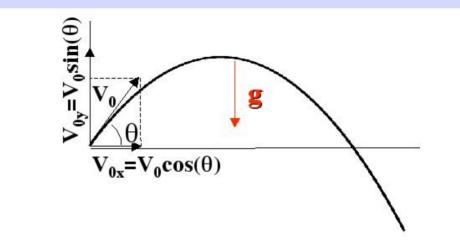
$$y = V_0 \sin(\theta) \left(\frac{x}{V_0 \cos(\theta)}\right) - \frac{1}{2} g \left(\frac{x}{V_0 \cos(\theta)}\right)^2$$
