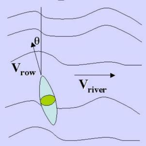
A person can row with speed V<sub>row</sub> in still water. In a river flowing at speed V<sub>river</sub>, at what angle should they row to go straight
