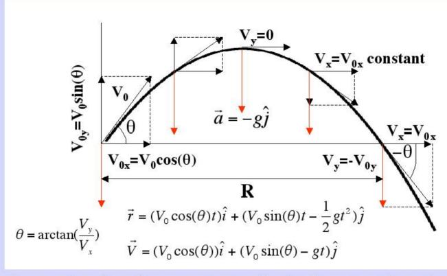
The motion in x has constant velocity because there is no acceleration in x.
