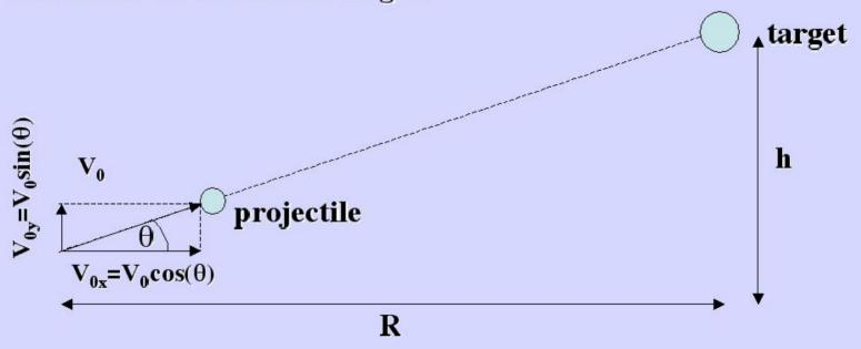
We can easily calculate components of the initial velocity and the time to the target given the distance R.
