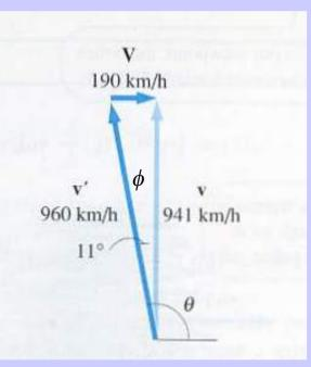
A Jetliner with an airspeed of 960km/h flies from Houston to Omaha, a distance of 1290km. The jetstream at altitude is a steady  $v_{js} = 190$ km/h from west to east. (a) In what direction should the jet fly?
