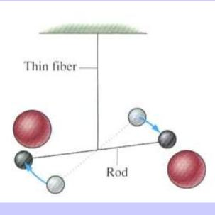
Astronomers measure the product *GM* for orbiting objects, but what about *G* itself? It is extremely weak but Cavendish found a way. He suspended two *5cm* diameter lead spheres connected by a thin rod on the end of a thin fiber. He then brought two *30cm* lead spheres close to the suspended lead spheres and measured the small rotation of the rod. Knowing the torsional property,  $\kappa$ , of the fiber, he was able to calculate *G*.
