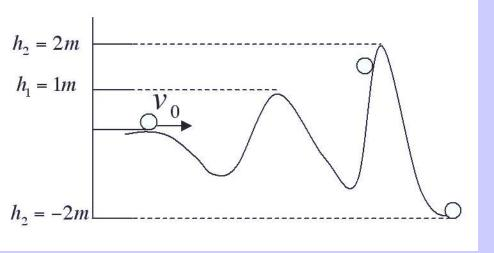
A ball is rolled onto the path shown. If its initial velocity is v = 6m/s what is the final velocity of the ball?
