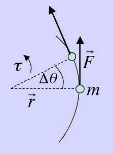
The K<sub>rot</sub> is as we expect, with I and ω analogs of linear motion. If we integrate the torque we find the work done in the angular acceleration, generating rotational kinetic energy:
