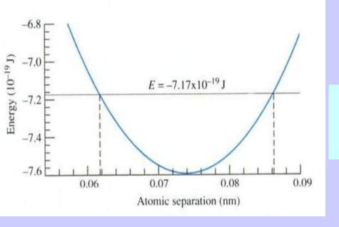
Near the bottom of the potential well,  $r = r_c$  the potential energy is given approximately by:
