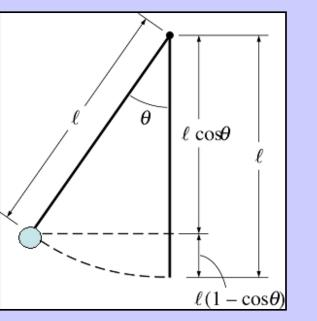
The Pendulum is one of the fundamental problems in mechanics. It can be used to understand many more complex problems in oscillatory motion. We will consider the simplest example.
