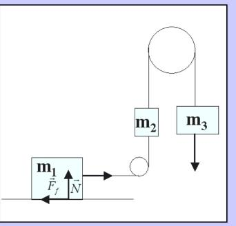
Three masses are attached to pulleys as shown. Mass  $m_1$  slides on a surface with a coefficient of kinetic friction  $\mu_k$ . Find the velocity, v, after starting from rest of the objects after traveling a distance  $\Delta y$ .
