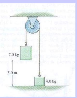
Consider the Atwood machine with masses,  $m_1 = 7kg$  and  $m_2 = 4kg$ . (a) Find the velocity of  $m_1$  just as it hits the floor. (b) Find the maximum height reached by  $m_2$ . (c) Find the fraction of the total mechanical energy lost when  $m_1$  hits the floor.
