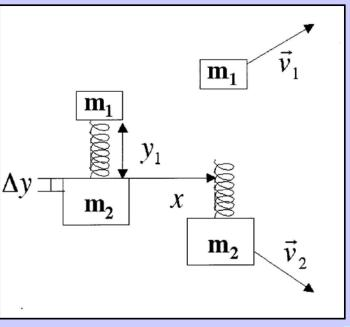
Two objects are moving in the *x* direction connected by a compressed spring in the *y* direction. Derive an expression for the velocities of the objects after the spring is released.
