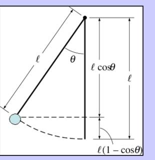
The Pendulum is one of the fundamental problems in mechanics. It can be used to understand many more complex problems in oscillatory motion. We will consider the simplest example.
