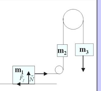
Three masses are attached to pulleys as shown. Mass  $m_1$  slides on a surface with a coefficient of kinetic friction  $\mu_k$ . Find the velocity, v, after starting from rest of the objects after traveling a distance  $\Delta y$ .
