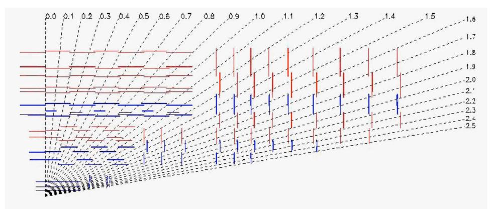
Figure 1.9: The tracker layout (1/4 of the z view).
