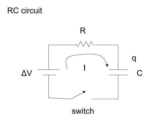
When the switch is closed how does the current and voltage change with time?
