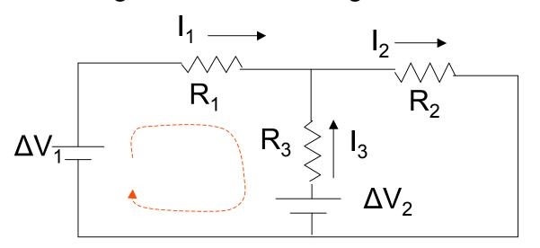
$$\Delta V_1 - I_1 R_1 + I_3 R_3 - \Delta V_2 = 0$$
