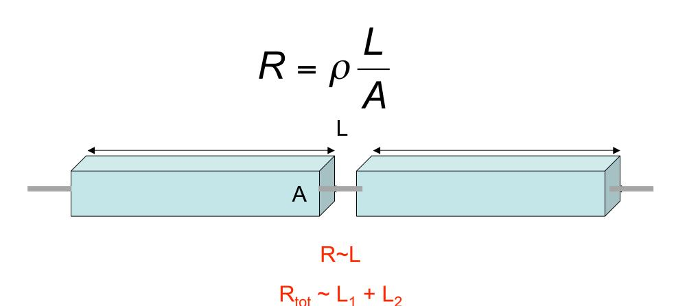
Resistors in Series I same,  $\Delta V$  different What is the equivalent resistance  $R_{eq}$ ?
