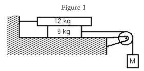
A system comprising blocks, a light frictionless pulley, and connecting ropes is shown. The 9 kg block is on a smooth horizontal table ( $\mu = 0$ ). The surfaces of the 12 kg block are rough, with  $\mu = 0.30$ .
