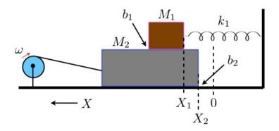
Figure 4.5: The equivalent mechanical circuit for fig. 4.4.
