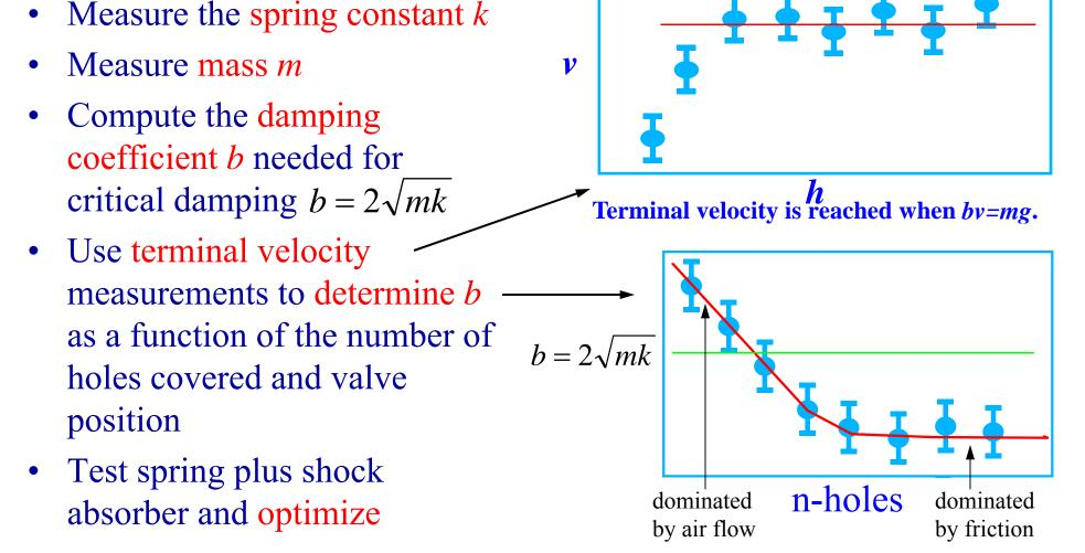
the valve is good for fine adjustment
