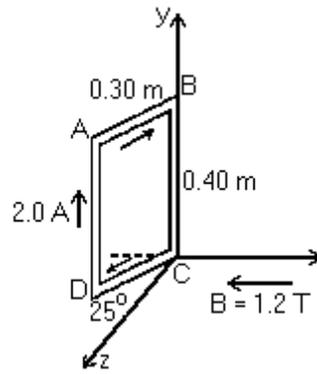
A rigid rectangular loop, which measures 0.30 m by 0.40 m, carries a current of 2.0 A, as shown. A uniform external magnetic field of magnitude 1.2 T in the negative x-direction is present. Segment CD is in the x-z plane and forms a  $25^\circ$  angle with the z-axis, as shown.
