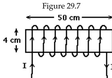
A solenoid is wound with 400 turns on a form 4 cm in diameter and 50 cm long. The windings carry a current in the sense that is shown. The current produces a magnetic field, of magnitude 1.5 mT, at the center of the solenoid.
